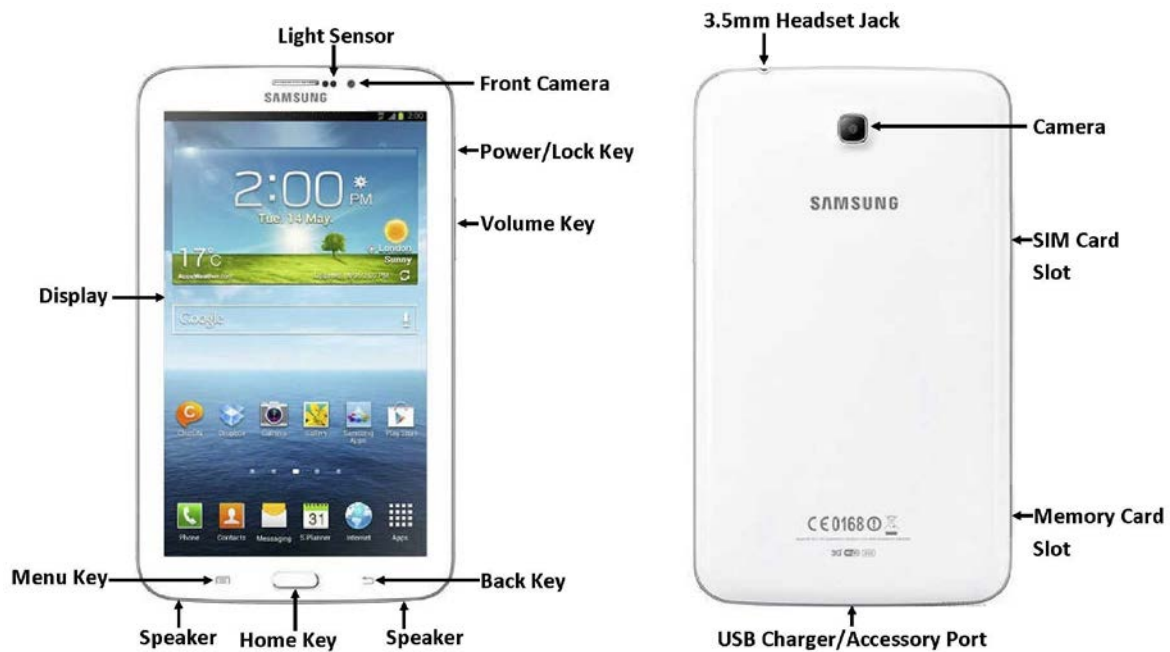
Figure 1 Parts of a tablet (Samsung Galaxy)
